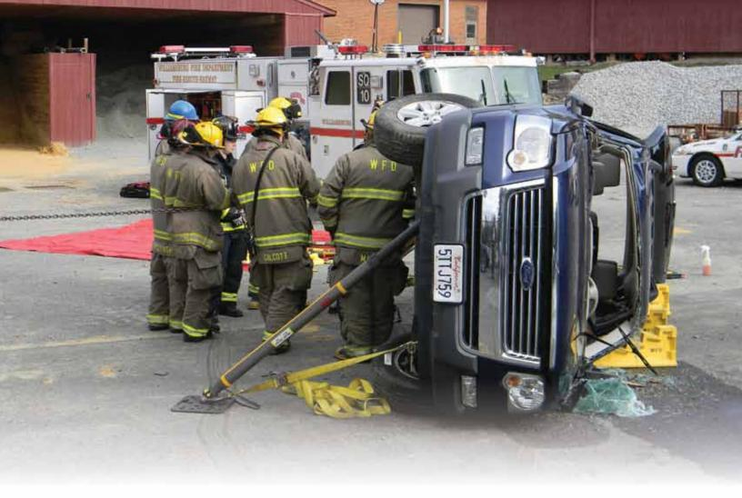
The City of Williamsburg Fire Department is now utilizing a vehicle stabilization kit in rescues where there is a potential for vehicle shift or rollover, to allow rescuers to focus on the extrication and treatment of passengers.
